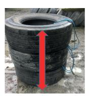
$2\ straps$  to be placed between the top tyre and tyre  $2\ (as\ per\ pictures)$  Straps can be of  $10mm\ rope$  or heavier doubled to make the loop
