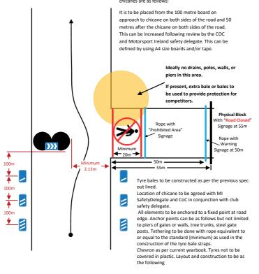
Tyre bales to be constructed as per the previous spec out lined
