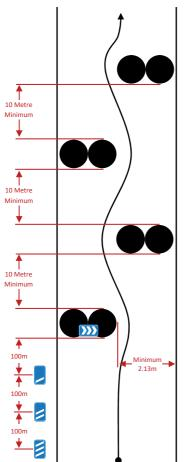
Ideally bales should overlap in order to block visibility through the chicane, though this is not always possible or necessary.
